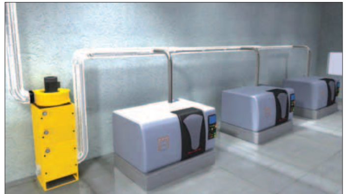
MistEliminator connected to three tooling machines
