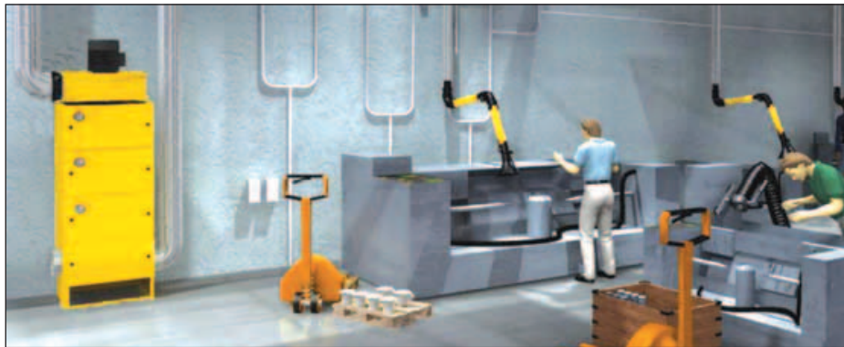
Source extraction arm system connected to MistEliminator
