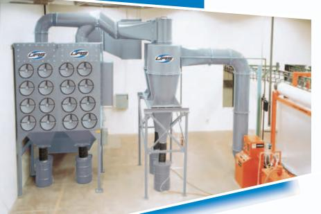
by means of the unit's long tapered cone, high-velocity inlet and welded helix. Dirty air enters the unit at a high speed and is then spun around in a spiral motion, throwing particles against its cone wall. Centrifugal force pushes the larger or heavy dust particles down through the larger or heavy dust particles and into a collection drum or hopper. Clean air runs back up the center of the unit, is discharged through the outlet and then exhausted back into the environment for safe breathing.
